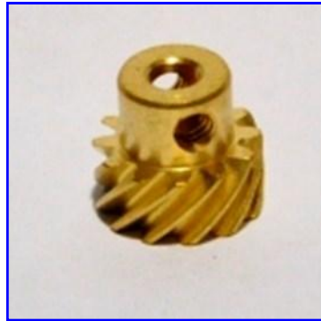
211d 12 tooth Helical, 2 of these give exact 1/2" spacing for 90 degree shafts.
