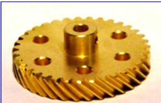
Pictured above 2 finished 60 Tooth RH Helicals.
