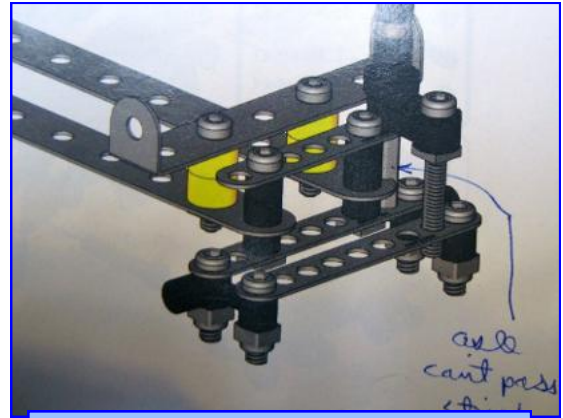
Mistake in instructions shows steering shaft passing through 1/2" wide chassis strip.
