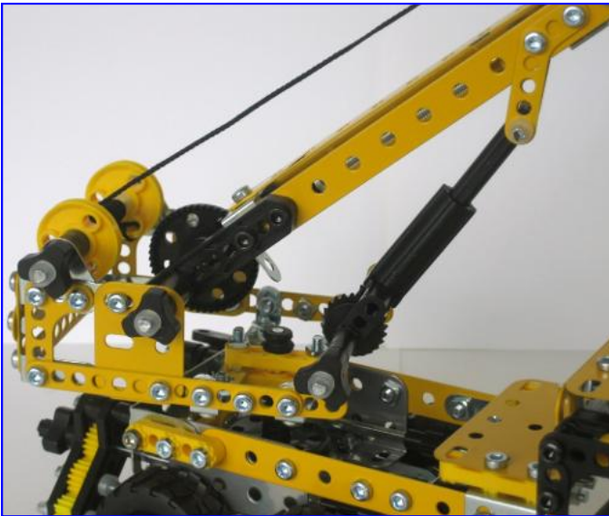
New plastic luffing cylinder and Bevel Gear.
