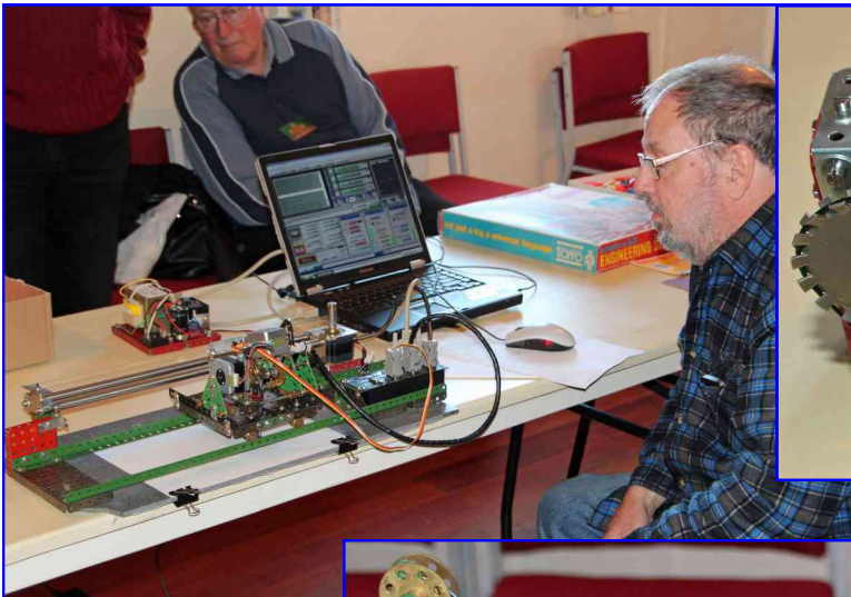
Richard Feltham's Meccano based 3D printer.
