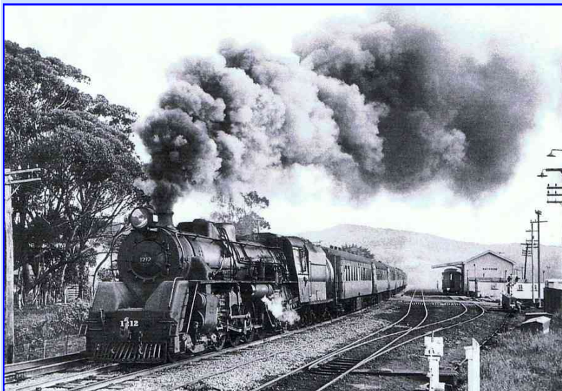
"J" Class No. 1212 built by the North British Locomotive Company, Glasgow in 1939 seen in almost new condition at the Frankton locomotive depot in 1940. Photo: J. Crebar collection.
