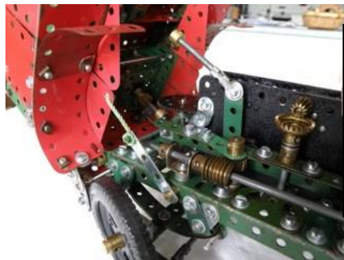
Cab tilted, showing cab stay, gear lever, motor output and steering drive.
