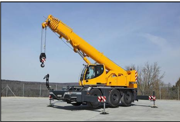
Figure 1: Prototype LTC 1045-3.1 Liebherr Compact Crane with cab moved back and elevated from its road travelling position. ( www.liebherr.uk )
