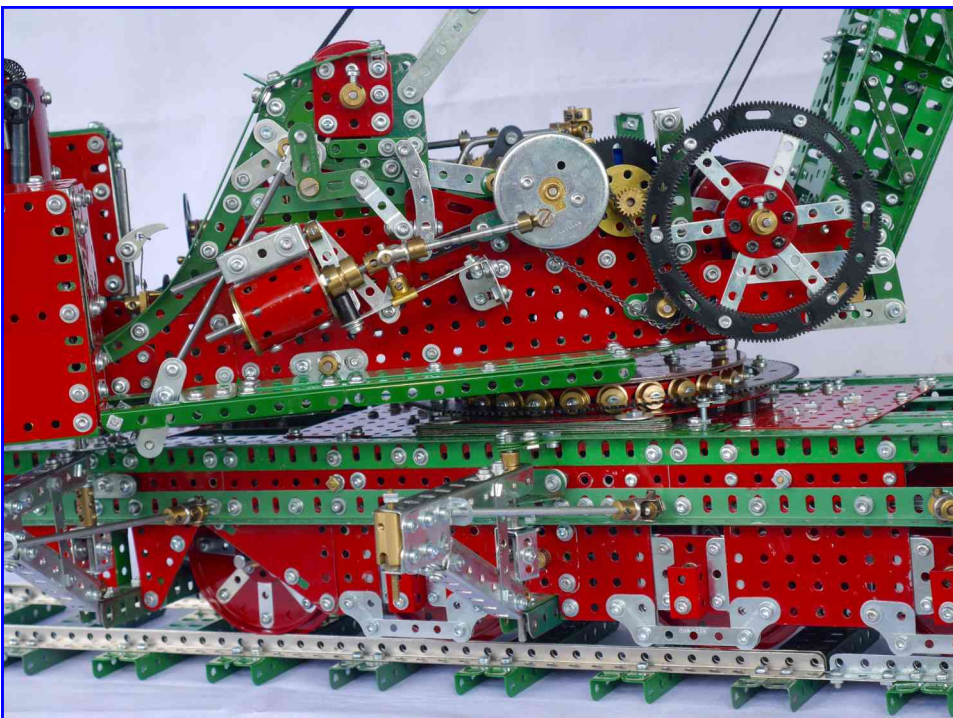
Fig. 2: Side view of crane frame showing cylinders and valve gear. The vertical lever at the back of the cab reverses the engine's direction. Two of the outriggers are in the propped out position.
