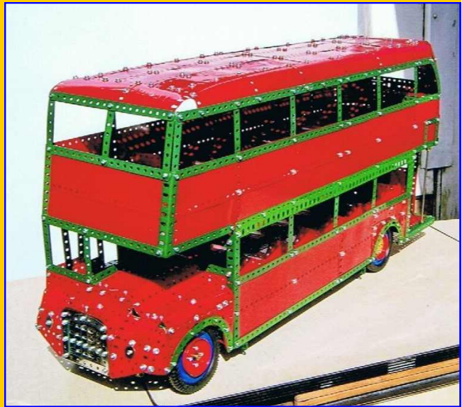
Double deck bus based on the No. 10 set leaflet (modified). Powered by 20V motor using leaflet's clutch, gearbox and differential. Not sure who the builder is. Barry says there is a need to strengthen the front axle because the body weight is causing distortion. The front of the bus was converted into a Routemaster.
