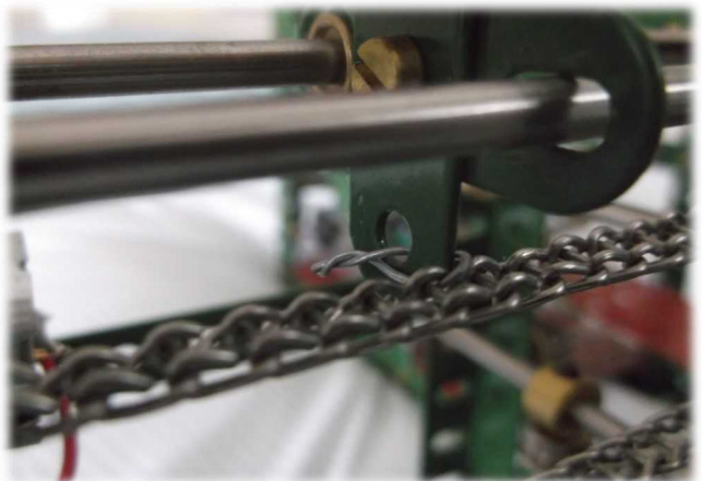
Figure 10 Another way of attaching a loop of chain to a sliding assembly
