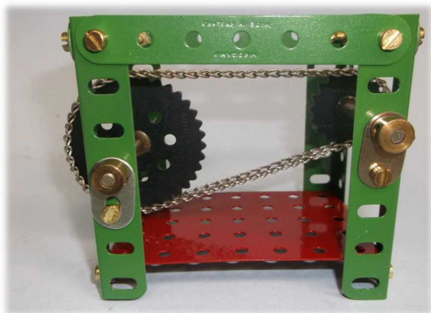
Figure 3 Axles supported in slotted holes, and the chain tensioned by adjustable fishplates. It may be possible and preferable to place the fishplates inside the angle girders.
