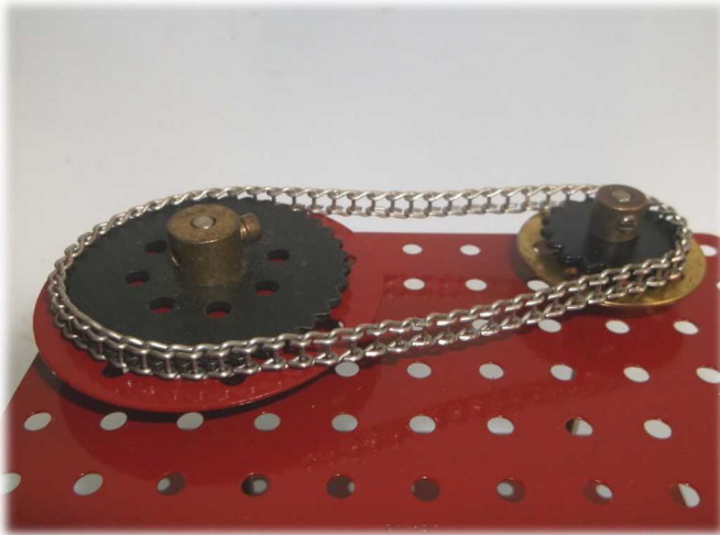
Figure 11 A loop of chain running in a horizontal plane, supported by a face plate and a bush wheel.
