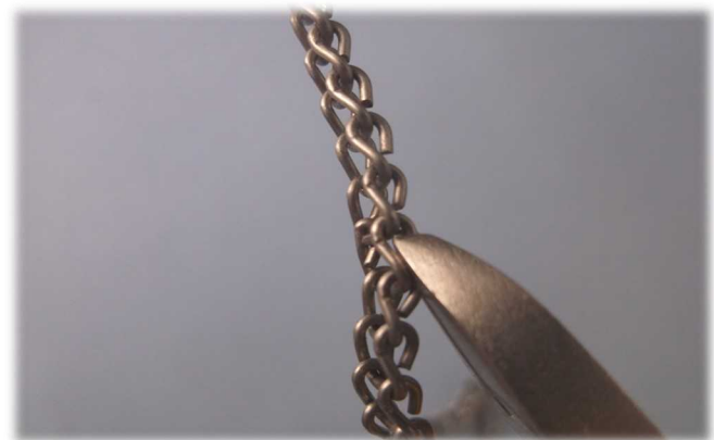
Figure 2 Opening a link of chain with side cutters
