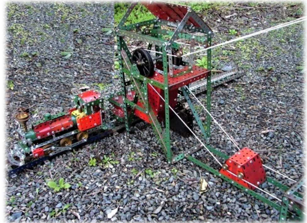
Fig 1: Detail of cable tensioner system
