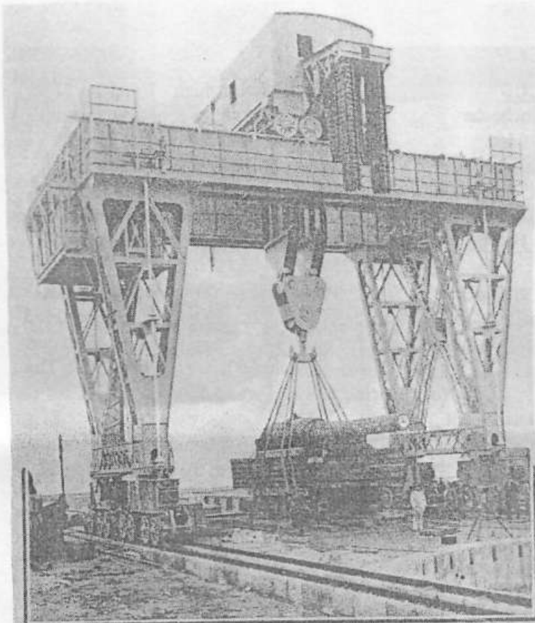
The 480-ton Gantry Crane lifting the barrel of a large calibre gun. The gun is placed on a wood plank platform in order to prevent any possibility of strain on the barrel.
